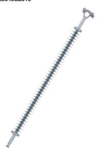
Line Post Insulator, 2.5" (63.5 mm) Rod Diameter, 21.9" Polymer Length, Standard Leakage Distance, Top Fitting: Tear Drop Blade, Bottom Fitting: 2-Piece Aluminum Gain Base, No Corona Ring
