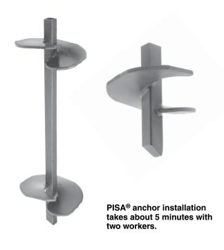
Chance Standard-Strength 4,000 foot-pound anchors and Mid-Strength 6,000 foot-pound anchors have curvilinear leading edges to help penetrate rocky soils and to reduce damage during installation. These anchors are available in single and twin-helix designs. The same installing wrench installs Standard and Mid-Strength anchors as well as Tough One® C10252- - series anchors. See page 4A-4 for installing wrench information.
