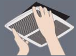
4. Install new grille
