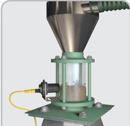
Pellet level detection - An 875CP detects the level of plastic pellets through a glass vessel
