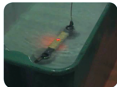
Actual Video Screen Captures of BW-223 During the Puncture Test. Note the corona on the outside of the test tank.
