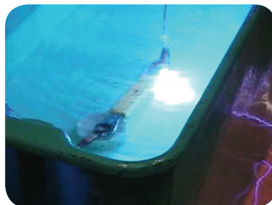
Actual Video Screen Captures of BW-223 During the Puncture Test. Note the corona on the outside of the test tank.
