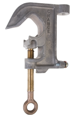
C6001743 Aluminum body, Smooth jaws, Bronze eyescrew with fine threads, Tapped for 5/8-11 UNC threaded ferrule
