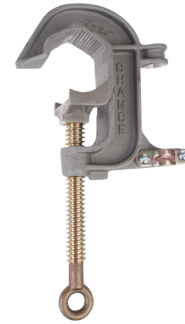
C6002256 Aluminum body, Serrated jaws, Bronze eyescrew with Acme threads, Tapped for 5/8-11 UNC threaded ferrule or PSC6003412, Drilled for 5/8-11 UNC threaded ferrule *Unshrouded Ferrules Only
