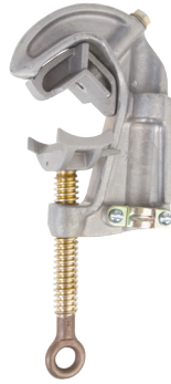
C6001733 Aluminum body, Smooth jaws, Bronze eyescrew with Acme threads, Tapped for 5/8-11 UNC threaded ferrule *Unshrouded Ferrules Only
