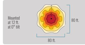
**Note:** Shown with a mounting height of 12 feet and 0° tilt All published photometric testing performed to IESNA LM-79-08 standards by a NVLAP accredited laboratory. Fixture photometry was completed on a single representative fixture.
