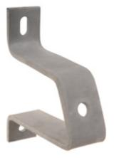
Post insulator bracket 9-1/2" long used for mounting distribution post-type insulators directly to pole. The base has a pole-shape back. Insulators not included. Has 13 /16" holes for stringing block.
