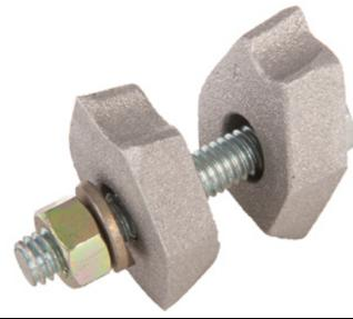
Thimbleye bonding clamp that fits 3/4" and 1" No-Wrench anchors. Bonding Clamps make a dependable mechanical and electrical pressure contact between guy strand and anchor rod, when the guy is part of the grounding system.
