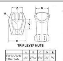
Pisa anchor rod 1" (25.4 mm) diameter, 3' 6" (1067 mm) long with Tripleye
