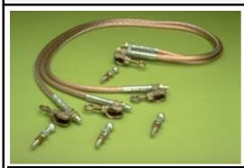
Each Ball-Stud set includes a three-way copper terminal block, four bronze ground clamps and three 6-ft. lengths of 2/0 copper clear-jacket ground cable with threadedstud aluminum ferrules. Ballstuds and clamps are C600-2102 and C600-2100.
