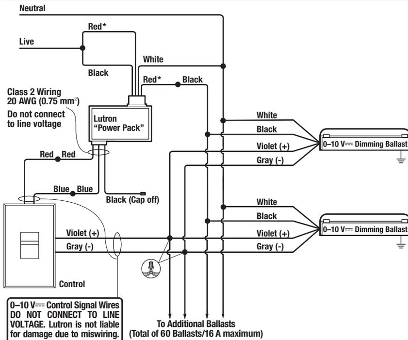
\* Red wires are interchangeable—either may be connected to line side or load side
