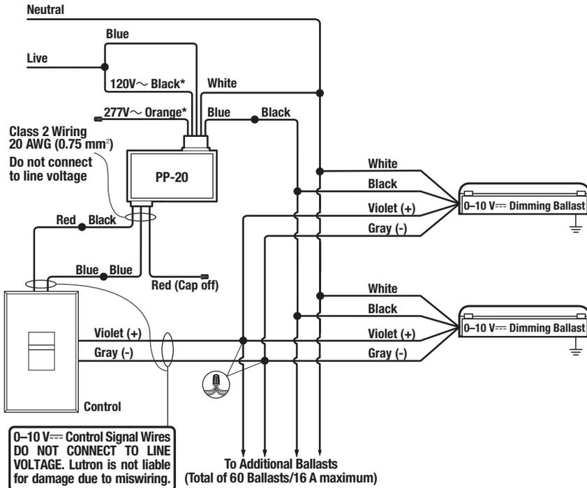
\* When wiring for 120 V~, cap off orange wire. When wiring for 277 V~, cap off black wire.
