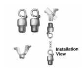
Complete assembly includes two hooks and one rigid support. Each hook supplied with a screw for closing 3/8" jaw opening. Rigid Support straddles max. 1-1/4" conduit. (Chain shown in installation view not furnished.)
