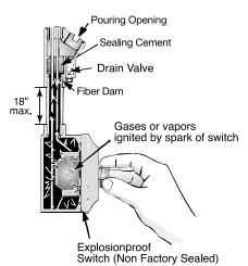
Appleton sealing fittings are suitable for Class I and II locations. EYS, EYSF and EYD are for sealing vertical conduit. EY and ESU are for sealing vertical and horizontal conduit. EYDM and EYD also have drain valves.
