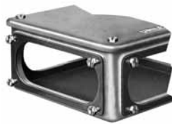
RS Box bottom and side frame construction is one piece malleable iron. Smooth hub cover openings prevent damage to conductor insulation.
