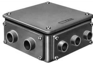
RS Box bottom and side frame construction is one piece malleable iron. Smooth hub cover openings prevent damage to conductor insulation.
