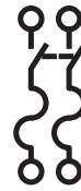
Fusible, Two-pole, 240 Volts AC; 250 Volts DC and Fusible Two-pole, 600 Volts DC, (2 poles in series for 600 Vdc)
