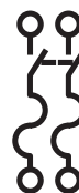
Fusible, Two-pole, 240 Volts AC; 250 Volts DC and Fusible, Two-pole, 600 Volts DC (2 poles in series for 600 Vdc)
