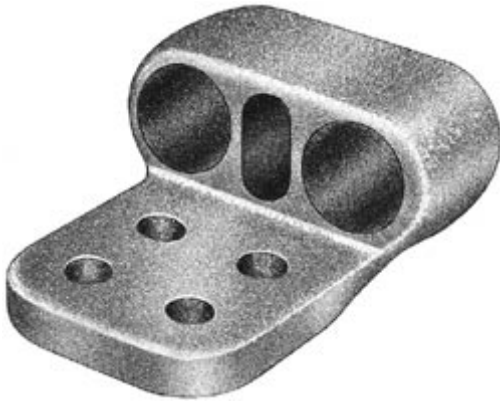
Terminal, Aluminum Weldment, Two Cables to Flat, cable range 1.263-1.315 Pad: 4 hole, 4 in
