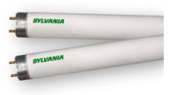
General32W, 48" MOL, T8 OCTRON XP Extended Performance fluorescent lamp,Description:6500k color temperature rare earth phosphor, 85 CRI, suitable for IS or RS<br/>operation, ECOLOGIC.
