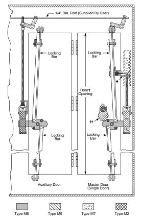
Interlocking lever extension of the flange mounted handle mechanism.
