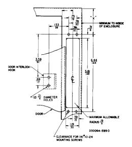
Panel Drilling for Alternate Mounting Method
