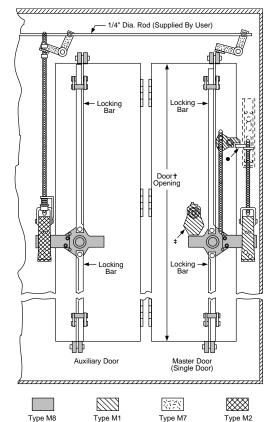
Interlocking lever extension of the flange mounted handle mechanism.
