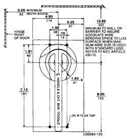
Panel Drilling for KAL, KCL, KHL Circuit Breakers and Operating Mechanisms
