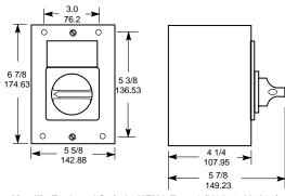
Metallic Enclosed Switch: NEMA Type 1 (V1G30, V2G30)
