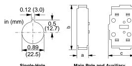
Single-Hole Drilling Dimensions
