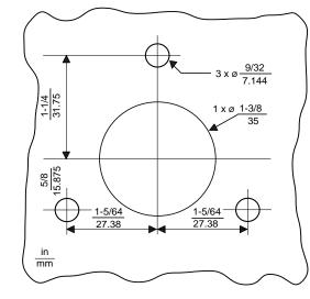
Panel Drilling for 9421 LC and LH Handles
