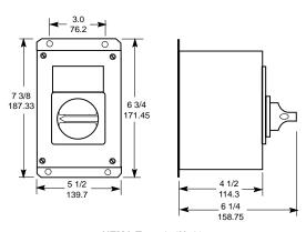
NEMA Type 4, 4X, 12 (V1W30, V2W30, V1A30, V2A30) **Class 9421**
