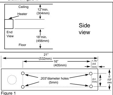
NOTE: The heater MUST be mounted horizontally to allow air flow freely upward through the heating element.
