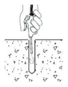
Tighten the anchor by turning the nut 3 to 5 turns past finger tight or by applying the guide installation torque from the finger tight position.
