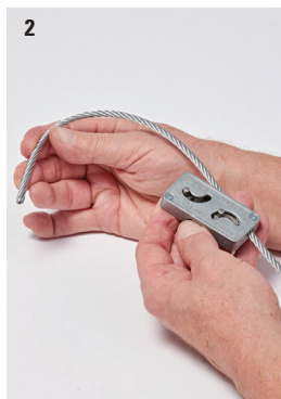
2 Loop wire rope through/around support
