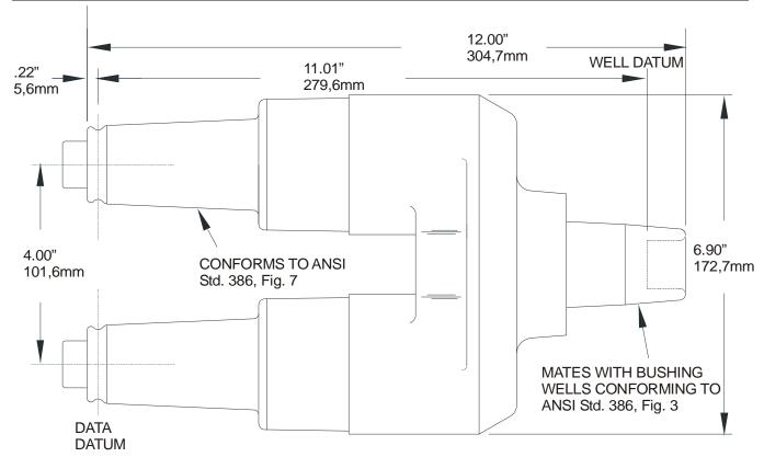
The Elastimold 2702A1 feed-thru bushing insert is fully rated with two 25kV class, 200 Amp load break bushing interfaces. The feed-thru bushing insert fits a standard ANSI bushing well interface and provide the capability of creating a tap position in an existing apparatus installation and transforming a radial-feed transformer into a loop-feed unit.
