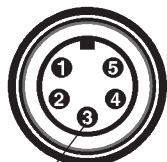
J1 Wiring Light Wired to N.C.
