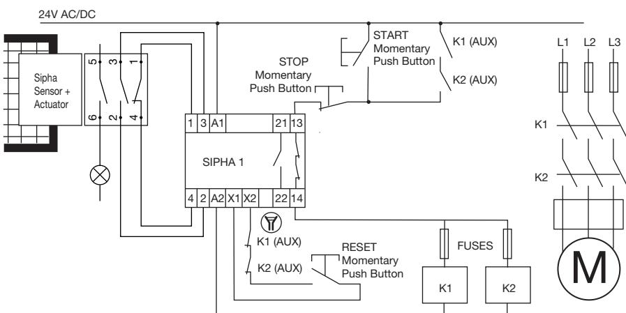
✿ Note: To energize outputs, at least one input must be closed after delay has expired.
