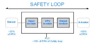
For the calculation of the PFD/PFH values of an example system, a maximum of 15% is assumed for the PLC. For the PFD/PFH values of the Quantum Safety modules, see *Available Safety Products, page 17*.
