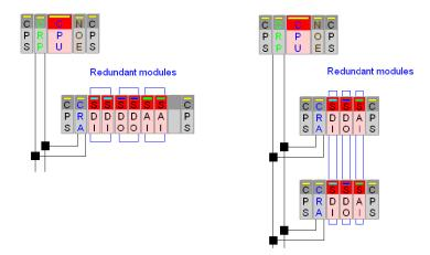
**NOTE:** Schneider Electric recommends always placing redundant Safety I/O modules in different RIO drops.
