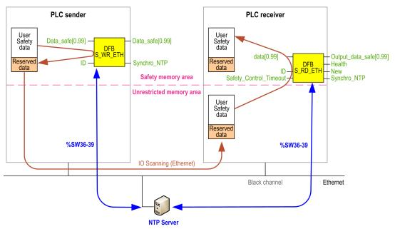
On the Ethernet network, you are allowed to mix safety related data and non safety related data without impact on the integrity level of the safety related data.
