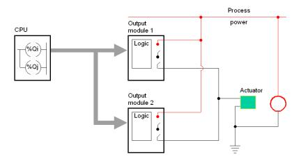
A function block is not necessary because the same signal from the CPU is connected to both outputs.
