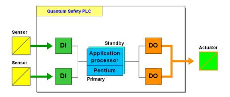
**NOTE:** Schneider Electric recommends always placing redundant Safety I/O modules in different RIO drops.
