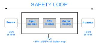
As shown in the figure above, the contribution of the PLC is only 10-20% because the probability of failure of sensors and actuators is usually quite high.
