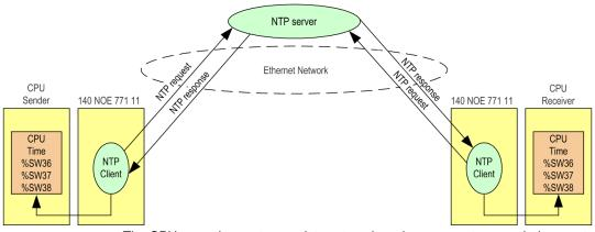
The CPU operating system updates at each cycle some system words (%SW36 to %SW38) that contain a time used by the safe communication as a time base. This time is internally filtered to avoid important time shifts and forbid fugitive bad values to be received from the NTP server.
