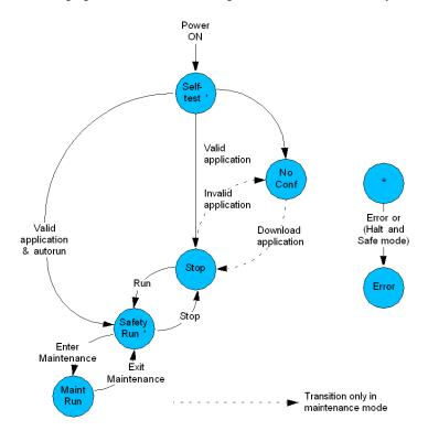
The following figure shows the state diagram of the Quantum Safety PLC:
