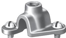
AL hangers can be furnished with a loop fastened to the top of the body to provide a means for suspending luminaires from vertical support rods or horizontal span wires. The loop will take a wire or cable with a maximum diameter of 3/8". The boss on top of the loop is tapped 3/8"-16 to accept a threaded rod.
