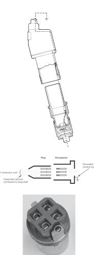
Style 1 Ground conductor attaches to shell.
