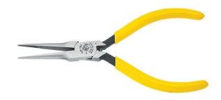
The knurled jaws on these 5-Inch Needle-Nose Pliers are designed to wrap and loop wire in confined spaces. These pliers feature a curved handle and sharp side-cutting blades for easy operation. Made of forged steel for maximum durability.
