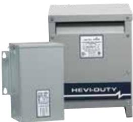
K-Factor Transformers are designed to reduce the heating effects of harmonic currents generated by loads such as variable frequency drives, power supplies and other electronic loads. The K-Factor rating is an index of the transformer's ability to withstand harmonic content while operating within the temperature limits of its insulating system. SolaHD K-Factor transformers have standard ratings of K-4, K-13, and K-20; other K-Factors are available as configured products.
