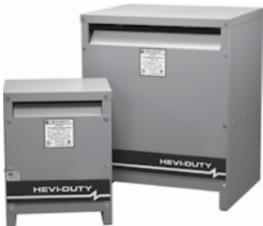
Low temperature rise transformers are designed for lower temperature rise in the conductors and core that result in longer life and better overload capability. All models available with either a 115°C or 80°C thermal rise and a Class 220°C insulation system.
