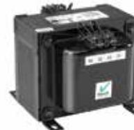
ICE International Series industrial control transformers are available from 50 to 2000 VA, 55°C or 80°C rise, and copper windings with epoxy encapsulation. Available with IP20 touchproof terminations, these transformers meet NEMA, ANSI and IEC requirements.
