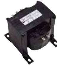
SMT Series industrial control transformers offer 115°C rise and aluminum windings, for applications where good voltage regulation and higher power capacities (1000-5000 VA) are required.
