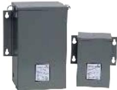
HSZ Series industrial control transformers are provided with a choice of UL Listed Type 3R, 4, 4X or 12 enclosures. Available from 1 to 10 kVA, 80°C rise, and copper windings. These fully encapsulated transformers provide protection from harsher environments, for reliable installation outside of a control cabinet. The HSZ Series is ideal for applications where cost or heat issues make mounting the transformer outside the control panel necessary.
