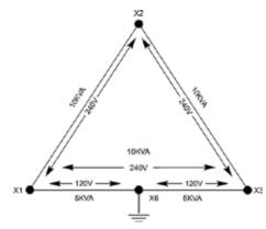
Note: All SolaHD 480 delta to 240 delta transformers stocked by Emerson are equipped with a center tap.
