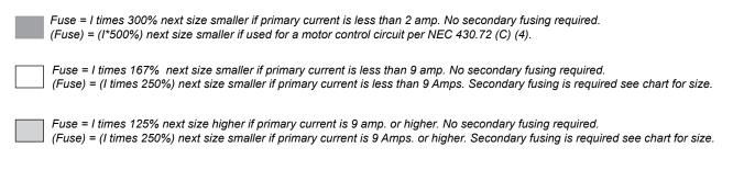
Recommended fuse sizes per UL 508 and NEC 450.3 (B), NEC 430.72 and commercially available type fuses.
