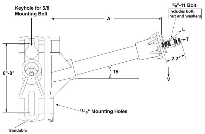
Base and End Fitting are aluminum alloy.
