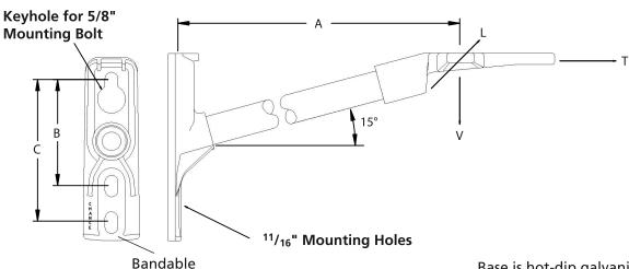
B Dimension is 6" C Dimension is 8" RUS Accepted. Base is hot-dip galvanized ductile iron and End Fitting is aluminum alloy.
