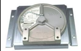
Turntable design permits proper alignment without repositioning service vehicle. Heavy-gauge steel base bolts direct to truck body wherever convenient. Bracket can be pinned at every 15° interval around circular base for stringing, tensioning, sagging conductors; pulling in cable; hoisting equipment; setting poles; pulling vehicles.
