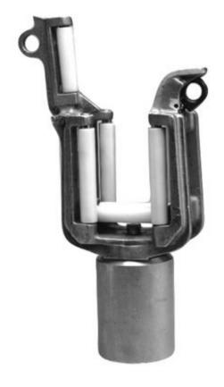
Seven Delrin plastic rollers offer protection to conductors while raising the conductor above the work area. Accommodates conductors up to and including 1.5 inches in diameter. The gate is held closed by a springloaded latch which must be manually opened.
