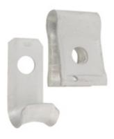
Figure 8 Cable Hanger, used to support integrated messenger wire. Accomodates .109" to .134" solid messenger wire. Clamp consist of two parts, "J" hook and the clamp. Installed with a 1/2" machine bolt and two square nuts (ordered seperately). One nut is placed between the hook and clamp for spacing and the other is used to tighten the clamp member.
