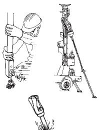
Attach anchor eye nut and the installation is complete
