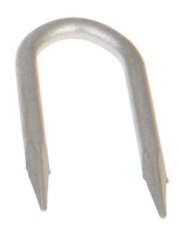
Diamond Point Staple, copper coated, 1" long x 1/4" inside width x .114" diameter wire. Used to secure ground wire and ground wire molding to wood poles.
