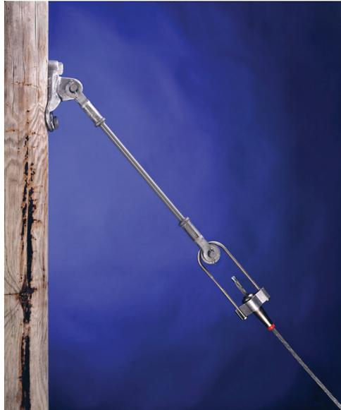
Chance Guy Strains use a veiled or optional silicone coated rod instead of a painted rod. These rods achieve high ultraviolet resistance while protecting the rod from surface scratches that would remove paint from other types of guy strains. Our castings are crimped (not glued) onto the rod and sealed with silicone for moisture lock-out. Prevention of moisture penetration at the rod/casting interface enhances the performance and life span of the guy strain.
