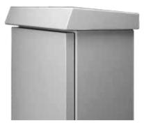
Solar Shield Top provides a vented area on top of the enclosure to absorb solar heating effects and help keep enclosure cool. Also provides a drip shield to keep liquids away from the door sealing surface. Aluminum with RAL 7035 textured light-gray finish inside and out. Maintains enclosure rating. Includes mounting hardware.
