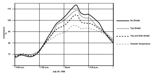
The results of the test show the enclosure with top and side shields to have approximately a 46% reduction in temperature compared to the unshielded enclosure. Hoffman offers top shields as an accessory for Hoffman COMLINE Wall-Mount Enclosures. The reduction in temperature is approximately 25% with the solar shield top only.
