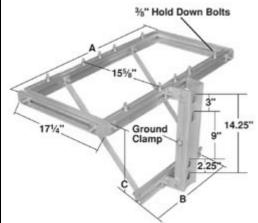
Aluminum Capacitor Rack, pole mounted, for mounting maximum 3 capacitors with 15 5/8" lug spacing weighing up to 80 lbs. each. Includes two pre-spaced 3/8" hold down bolts, flat washer, lockwasher and nut per capacitor mounting position and a ground wire clamp secured with 3/8" bolt. Supplied factory assembled and ready for installation of capacitors.
