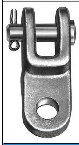
Clevis Eye, Rotated, Ductile Iron, Clevis: 1.000" Opening, 0.750" Pin, Eye: 0.750" with 0.688" Hole, UTS 36,000 lb
