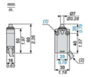
(1) 2 fixing holes  $\emptyset$  4.2 mm, counterbored  $\emptyset$  8 mm by 4 mm deep.
