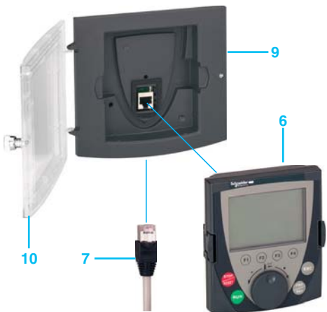
Remote location of the graphic display keypad on enclosure door: 6 + 7 + 9 if IP 54, 6 + 7 + 9 + 10 if IP 65
