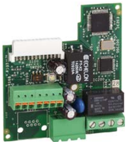
LonWorks communication card VW3 A21 212
