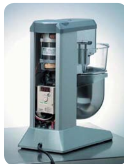
Application of an ATV 12 in a mixer
