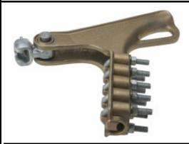
Strain Clamp, Quadrant, Heavy Duty, Bronze, Conductor Range 0.3 - 0.68 in, Fitting: Socket
