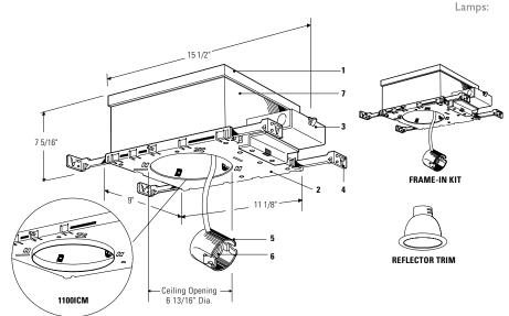
Complete Fixture consists of Reflector Trim & Frame-In Kit. Select each separately.
