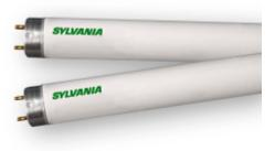
General25W, 36" MOL, T8 OCTRON fluorescent lamp, 3500K color temperature, rareDescription:earth phosphor, 82 CRI, suitable for IS or RS operation, ECOLOGIC
