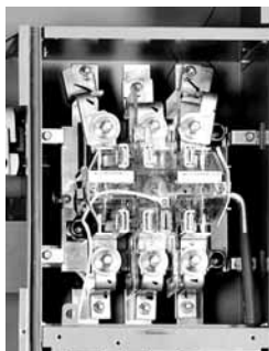
225 A Ringless-Type Meter Socket, Seven-Jaw with Lever Type Bypass Shown with Lexan Shield over Line and Load Meter Jaws
